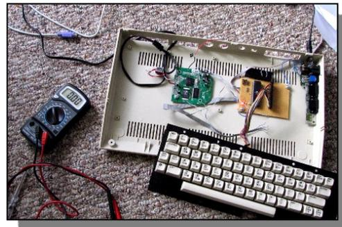
A - Some. The original design itself is quite strange. The keyboard membranes have some resistances (65-75 ohm), but there is no protecting diodes on the CIA lines, therefore it's possible to make a short circuit if one row drives Vcc while the other does Gnd and you press two keys in the same column.
