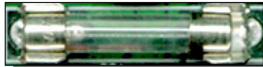
test it with a multimeter or take it to an electrical specialist for a replacement they should be only a few U.k. pence, i was charged 10 pence for a replacement, and the guy in the shop even kindly tested it for me. See the how to use a multimeter for continuity testing section.
