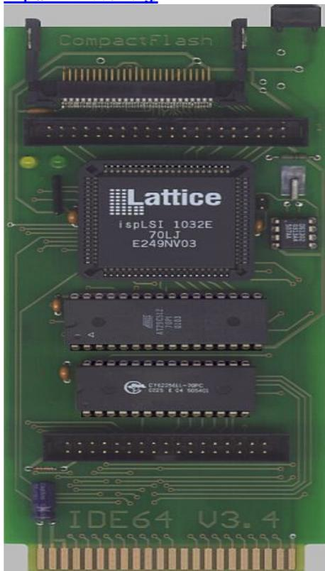
The ide 64 is a cartridge that allows standard pc IDE disk and cd rom drives to be connected to your Commodore, although it seems everyone is sold out there is a new version in the making see this link for more details <http://www.ide64.org/ide64v4.html> There is a patch for Geos to work with the device to my knowledge Wheels doesn't support the system. If you are a games fan you can copy most single file games on the device and load them very quickly
