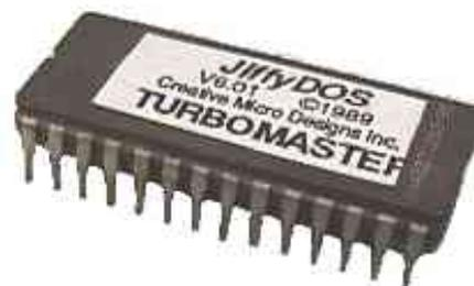
Jiffy dos is a floppy drive speed up system the chip needs fitting in the Commodore machine and also in your drives for the device to function to its potential, but as the ram link SCPU and FD drive have jiffy dos already installed, you could add a SCPU and a FD200 disk and be jiffy dos enabled, although other disk drives will need the chip fitted to take advantage
