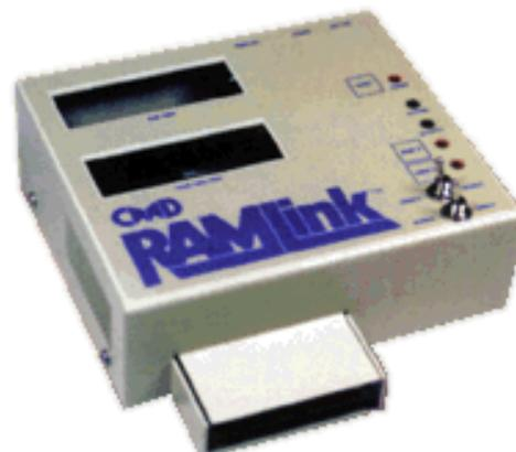
Can feature upto 16mb of memory is super cpu compatible ie they can work together allows the user to set up partitions to have disks instantly accessed, also features a battery backup to save the partitions when the device is powered off
