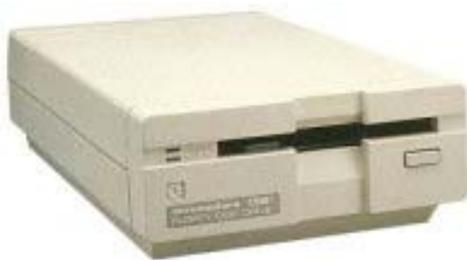
The 1581 is a floppy disk drive but uses 3.5 inch single density disks these are more readily available than the 1541 5inch disks
